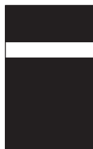
White bands in main scan direction
