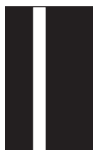
White bands in sub scan direction
